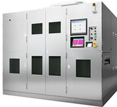
A direct imaging system for printed-circuit boards
