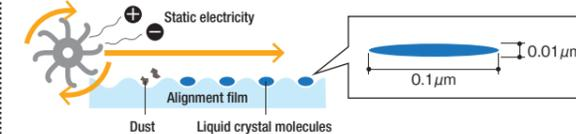
Yield suffers due to fine dust (particles) and generation of static electricity. The special cloth used for rubbing is not only expensive, but must be frequently replaced, increasing production cost and lead time.
