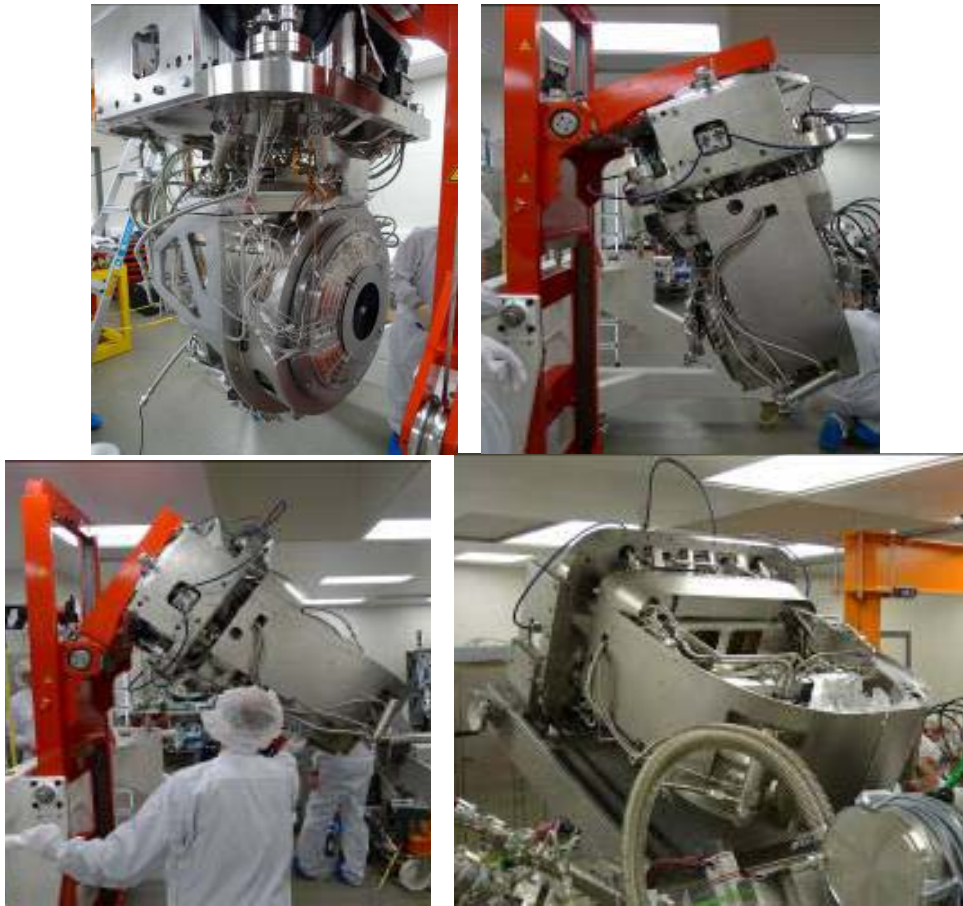
figure 7 Image sequence during the exchange of the swap flange containing the foil trap and the collector optics.
