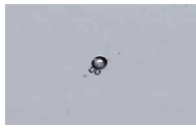
Bubbles in the glass ※ Bubbles are enclosed in the glass and have no impact on quality.
