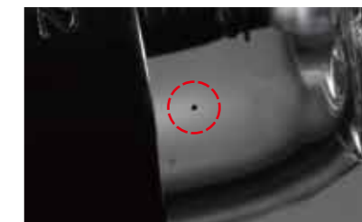
Foreign particle attached on the bulb ※ Some materials, etc. used in the lamp may adhere to the side bulb during the manufacturing process, but have no impact on quality.
