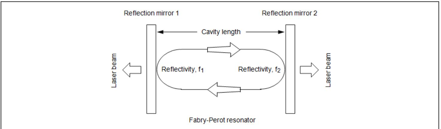
**Figure 3 Fundamental Structure of Fabry-Pérot Resonator**
