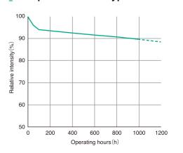
※9 Horizontal luminous intensity at continuous use. Frequent switch may cause shorter life.
