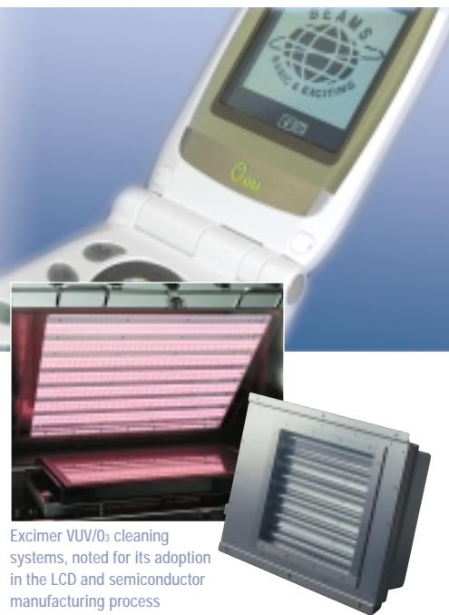
Excimer VUV/O<sub>3</sub> cleaning systems, noted for its adoption in the LCD and semiconductor manufacturing process
