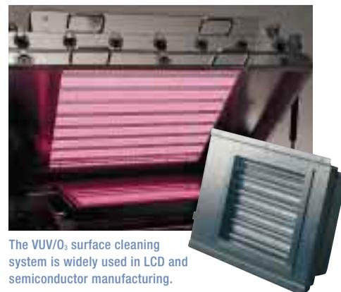
The VUV/O<sub>3</sub> surface cleaning system is widely used in LCD and semiconductor manufacturing.
