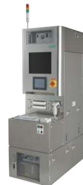
Mask/pellicle defect detection system
