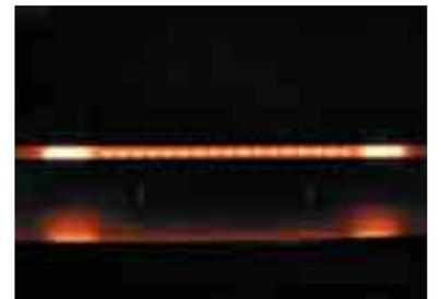
Multifilament Heater® when lit (The central part is set at a lower temperature while both ends are set at a higher temperature.)
