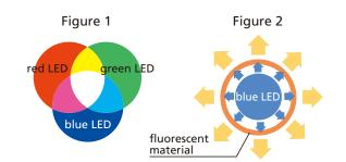
The development of a blue LED made it possible to create natural, "white" light by combining the three primary colors of light (Figure 1). Another method of creating "white" light is to shine blue LEDs onto a fluorescent material, which then emits the full spectrum of light (Figure 2). Both methods are used, for differing applications.
