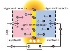
This structure can be used in reverse, by solar power cells, to generate electricity. By shining light on the chip, the positive and negative charges accumulate in the light-emitting layer and can be connected to a power circuit.
