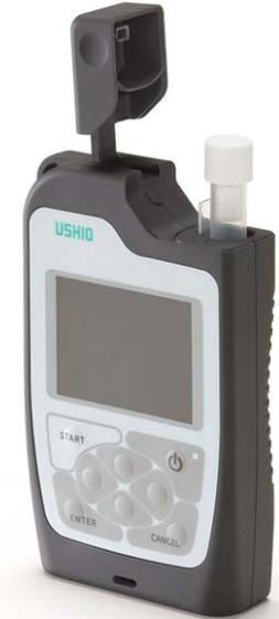
Onsite microanalysis kit which allows detection at a nanogram level. It can measure the target in 90 seconds through 3 steps.
