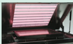
Excimer irradiation units for cleaning panels
