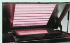
Excimer irradiation units for cleaning panels
