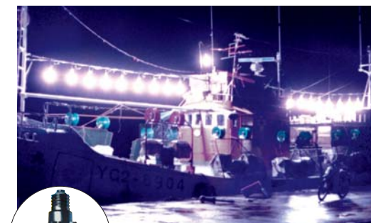
Halogen fish-luring light Introduced in 1973, this was Japan's first fish-luring light to use a halogen lamp. Twice as bright, lasts five times as long, and one tenth the size.
