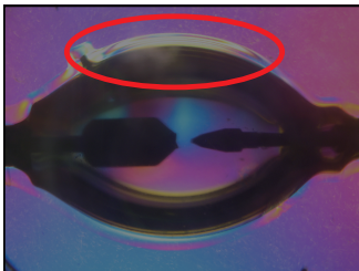
Figure 1. Distortion observed using sensitive color process. The colors appear different due to the changes in refractive index of stressed parts.
