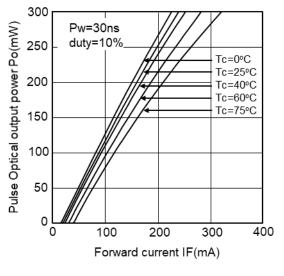
Pulse Optical Output Power vs. Forward Current
