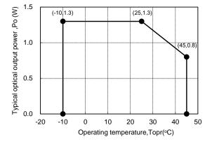
Fig.1 The relation of optical output power vs operating temperature
