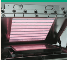
Panel photo-cleaning equipment
