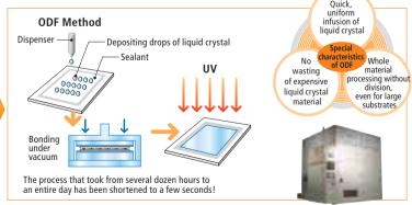
UV curing equipment for bonding LCD panels
