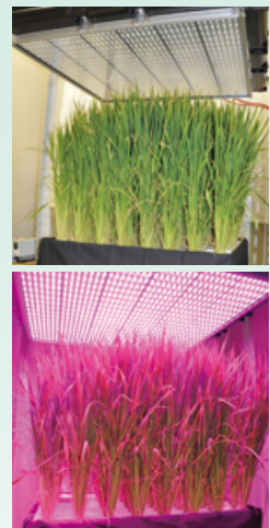
Rice is bathed in light from USHIO’s high-output LED units. This trial is the first time in the world that grain has been grown under artificial light.
