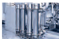
(1974) UV water sterilization system A UV water sterilization system using an inbuilt low-pressure UV lamp
