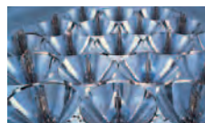
(1975) Large-scale solar simulator for testing satellites Delivered to the National Space Development Agency of Japan (currently the Japan Aerospace Exploration Agency) Also participated in the Japanese government's Sunshine Plan
