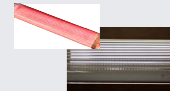
Prototype reactor that uses light to instantaneously decompose low-concentration N 2 O and CH 4
