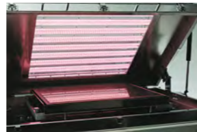
Excimer irradiation units for cleaning panels
