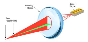
The diagram above illustrates the problems of astigmatism, and how it can limit your optical system performance in terms of focused beam shape and size. If precise beam placement or a small, focused image is required by your system, correcting astigmatism will improve your system performance.
