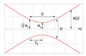
$\label{eq:searchine} \begin{array}{l} b = Beam \mbox{ Waist Depth of Focus} \\ W(z) = Beam \mbox{ Radius} \\ W_0 = smallest \mbox{ possible beam radius at focal point} \\ Z_R = Rayleigh \mbox{ length (distance from $W_0$ to edge of beam waist focus)} \\ Z = direction \mbox{ of beam propagation} \\ \theta = Beam \mbox{ divergence angle} \end{array}$
