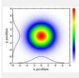
Mini*Lase*<sup>TM</sup> products often utilize our microlens ( $\mu$ lens<sup>TM</sup>) technology to gain distinct performance advantages over traditional laser diode based modules using anamorphic prism pairs or beam circularizing apertures. The  $\mu$ lens<sup>TM</sup> technology transforms a standard laser diode's elliptical beam profile and astigmatism into a Gaussian-circular beam profile with corrected astigmatism with no power loss.
