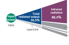
Visible radiation 7.1% Terminal loss 1.5% Glass/base absorption 5.0%
