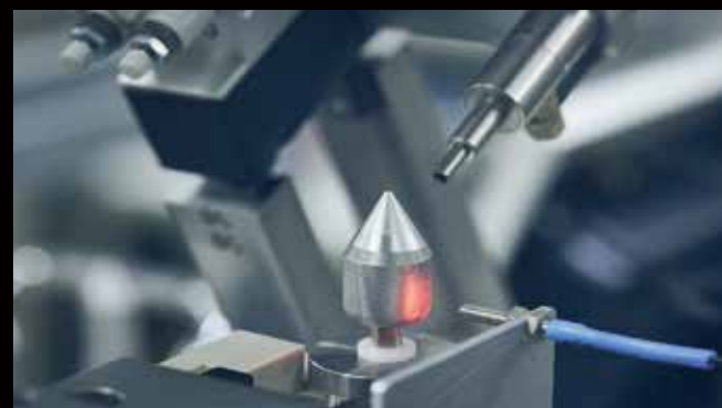
Automated inspection of cathode surface finishing
