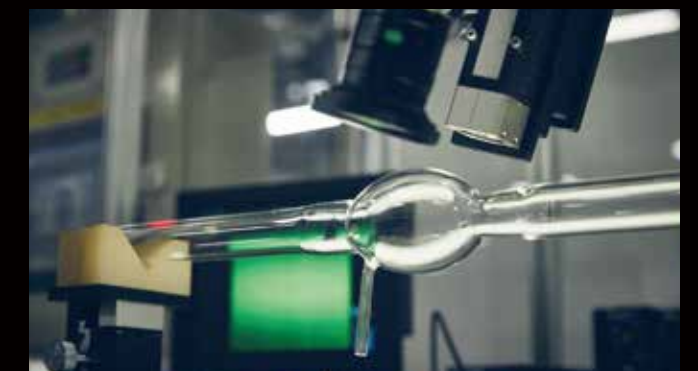
Automated inspection of bulb shape
